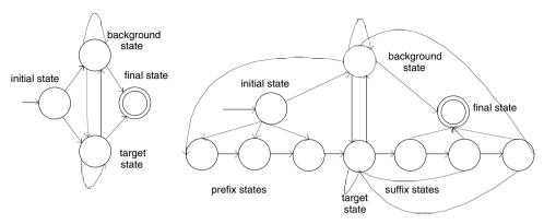
Figure VIII.1. Possible topologies of a simple HMM.
