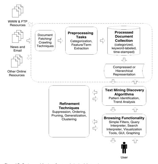
Figure I.5. System architecture for generic text mining system.
