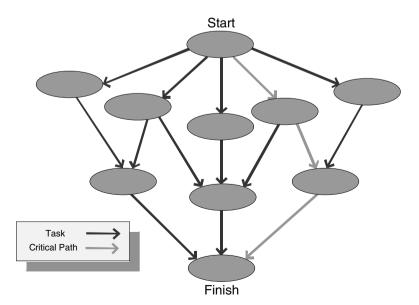
Figure X.36. Critical path diagram.
