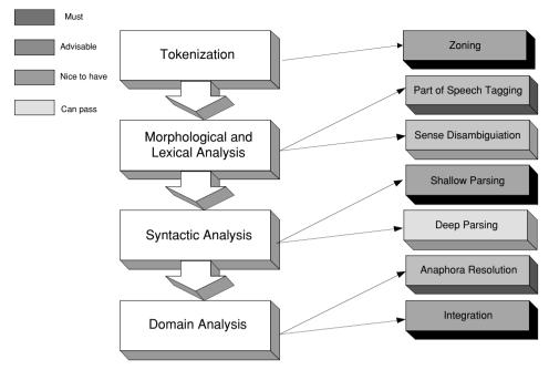
Figure VI.5. Architecture of a typical information extraction system.
