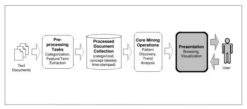
Figure X.3. High-level functional architecture of a text mining system showing position of visualization.
